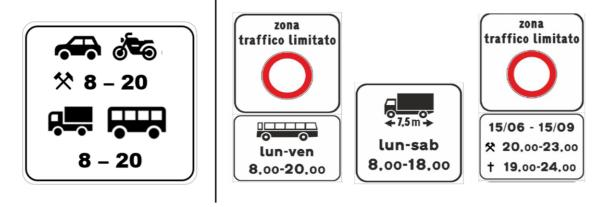
Figure 14: Supplementary panels for time validity, examples from France (optimised - left), and Italy (existing vs. optimised - right).
